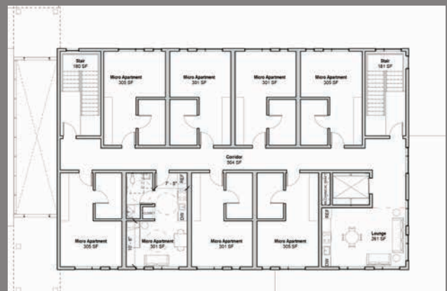
Micro Apartments, Second Floor of Common House
